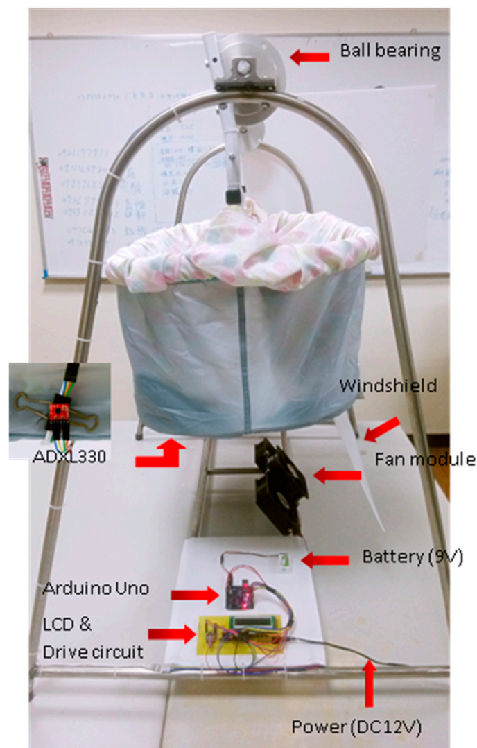
Figure 2. A resonant cradle design using wind power.
