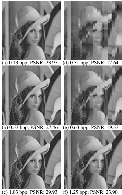
(a) 0.13 bpp; PSNR: 23.97 (d) 0.31 bpp; PSNR: 17.64 (b) 0.53 bpp; PSNR: 27.46 (e) 0.63 bpp; PSNR: 19.53 (c) 1.03 bpp; PSNR: 29.93 (f) 1.25 bpp; PSNR: 23.90 Fig. 3. The first three phases of “Lena” using BWPIT (a)-(c) and the corresponding phases using WbPIT (d)-(f)
